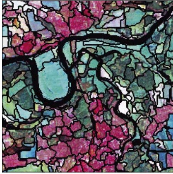
Fig. 3: segmentation of a LANDSAT scene with optimization of spectral homogeneity together with shape homogeneity
