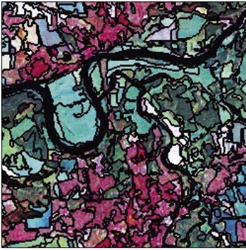
Fig. 2: segmentation of a LANDSAT scene with exclusive optimization of spectral homogeneity
