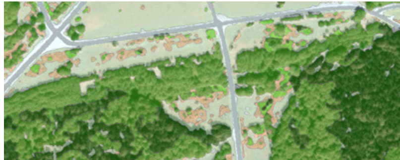
A subsection of the eCognition classification. IABG integrated LiDAR-derived DEMs, optical satellite imagery, aerial photos and other data into eCognition to distinguish Blackthorn from other vegetative types. There was not a single mismatch between what eCognition classified as Blackthorn (including its varying heights) and what was on the ground.
